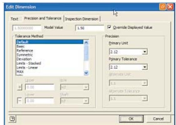
**Copy Dimension Properties**—similar to the AutoCAD Match Properties command, the new Copy Properties tool provides a quick and easy way to select a source dimension and apply its properties to other dimensions.
