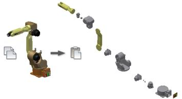
The enhanced copy and paste operation produces a duplicate of the copied components with connections and orientation intact.
