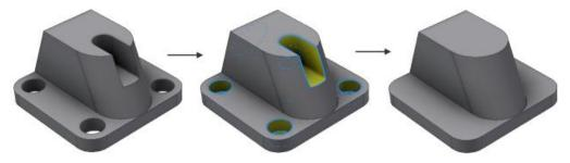
**Define Envelopes** Simplify a model by replacing selected components with box/cylindrical envelopes or creating simple extrude features that represent their shape.
