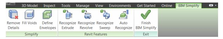
Remove Details Simplify a model by removing recognized fillets, chamfers, or custom-selected faces.
